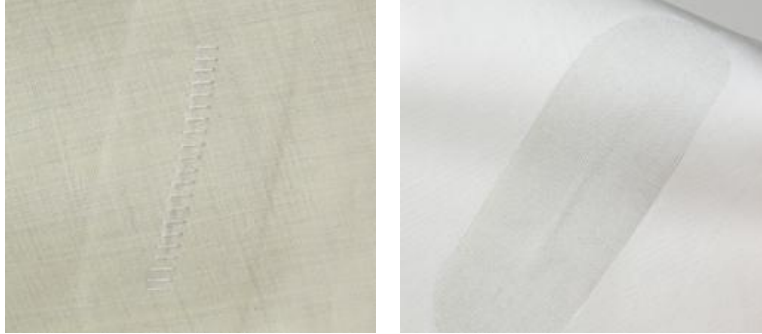
Sew-and-tape repair for straight tears
